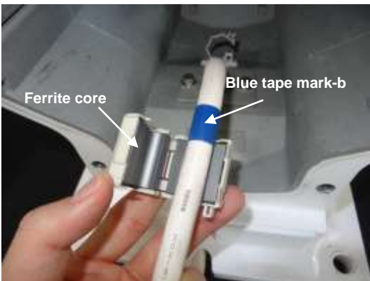
11) Attach the ferrite core to side of the blue tape mark-b.
