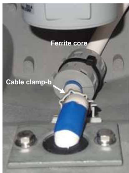
14) Clamp the cable by the cable clamp-b.
