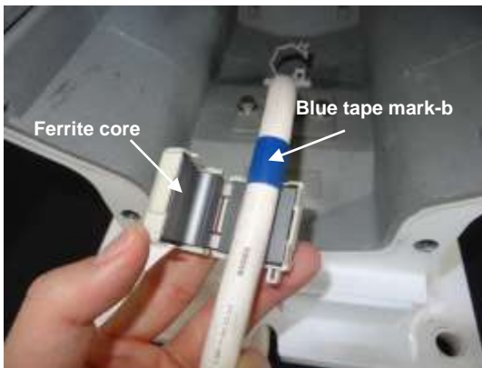
11) Attach the ferrite core to side of the blue tape mark-b.
