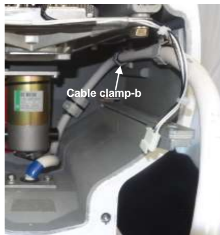
14) Clamp the cable by the cable clamp-b.
